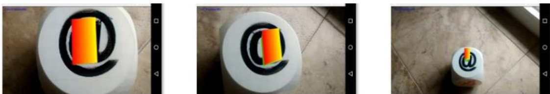
Figure 5: Qualitative results of the Augmented Reality prototype. A simple 3D object is overlaid on a real object. Performance decreases with capture scale of the real object.
