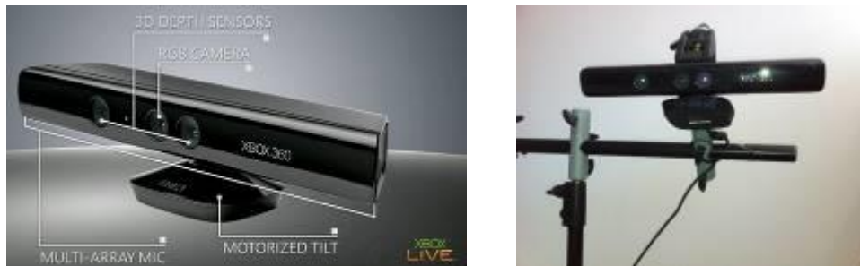
Figure 8 Detail of a Kinect camera and its placement.
