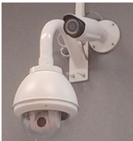
Figure 1. Cameras positioning. The cameras are placed 5 metres over the floor level
